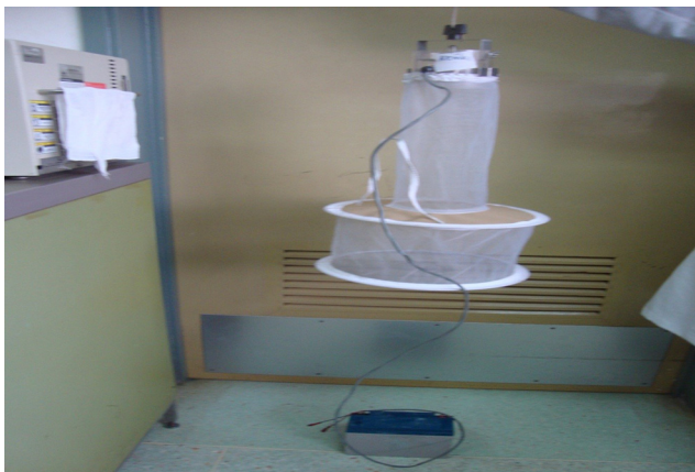
PHOTO 2. A CDC light trap set inside a house to trap mosquitoes seeking a host indoors.
