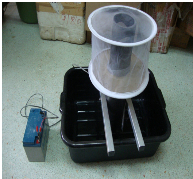
PHOTO 3. A CDC gravid trap set inside a house to trap mosquitoes seeking a host indoors.
